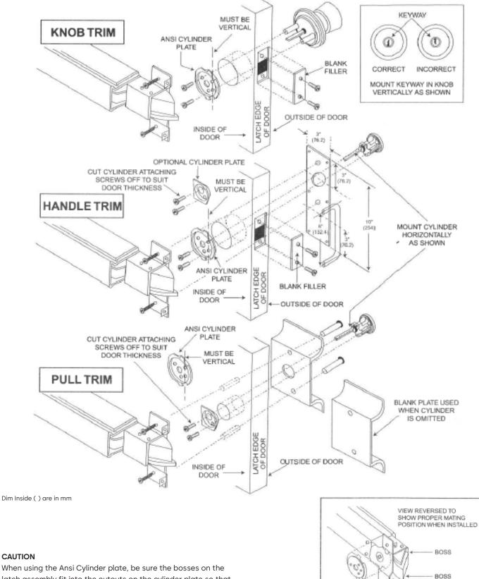
latch assembly fit into the cutouts on the cylinder plate so that the latch assembly lies flat on the door.
